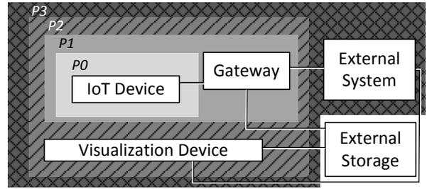
Fig. 1. IoT System Architecture and Security Perimeters (P0,P1,P2,P3)
