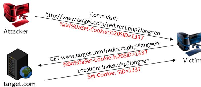
Figure 2: A Header Injection Attack
